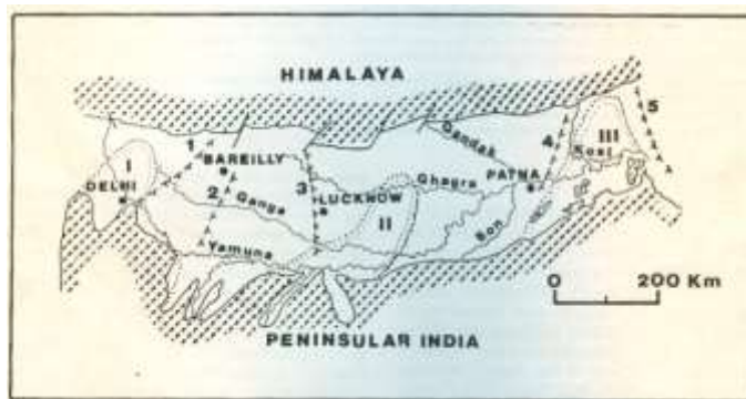
Figure 3.1: Sketch map of Gangetic plain showing position of major basement structures below the alluvium. I. Delhi ridge, II. Faizabad Ridge, III. Monghyr-Saharsa Ridge. 1. Moradabad fault, 2. Bareilly fault, 3. Lucknow fault, 4. Patna fault, 5. Malda fault. Based on data of Sastri et. al. (1971), and Rao (1973).
