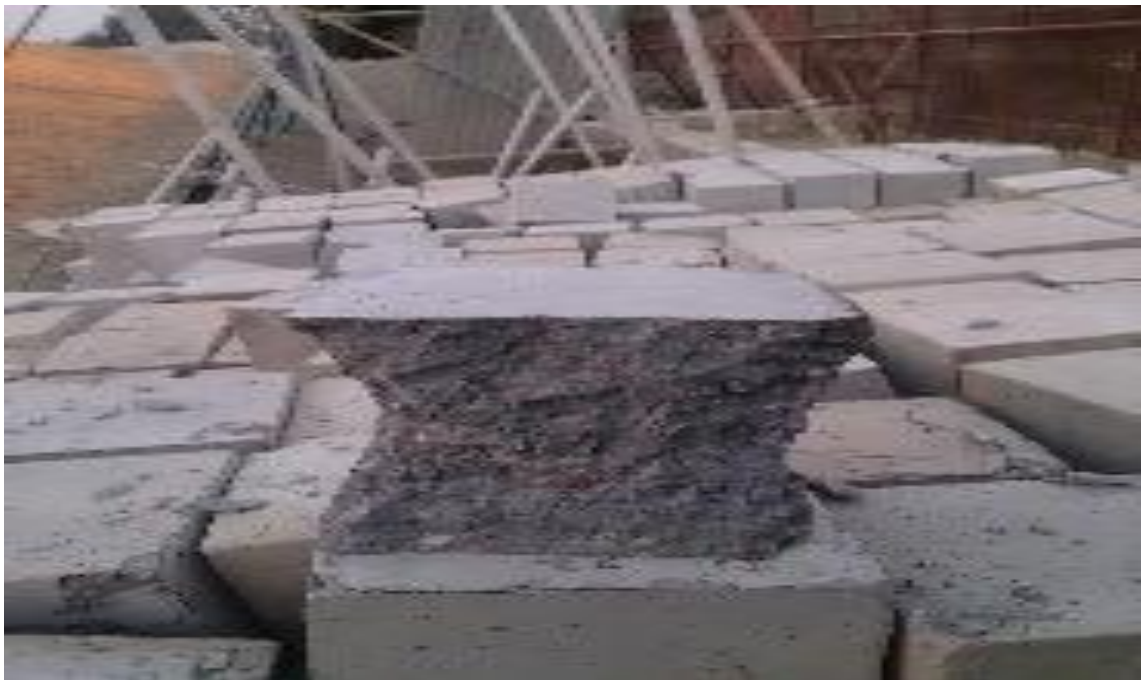
Fig:4.10 Concrete Cube After Failure
