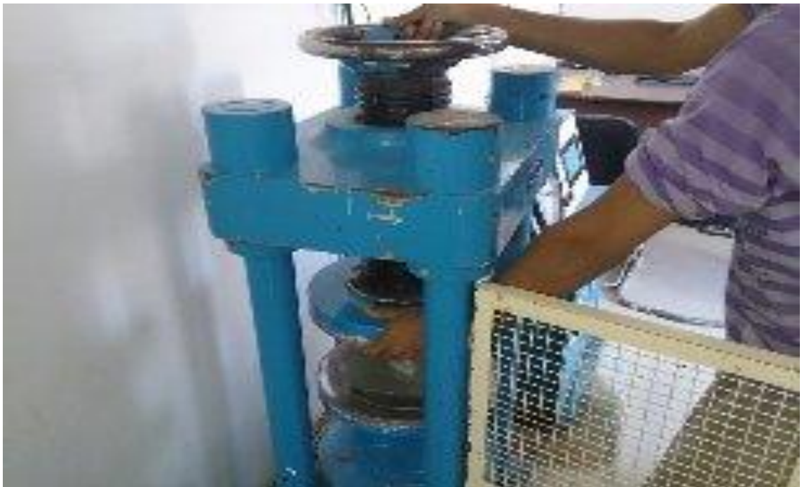
Fig:4.11 Placing of Specimen in CTM
