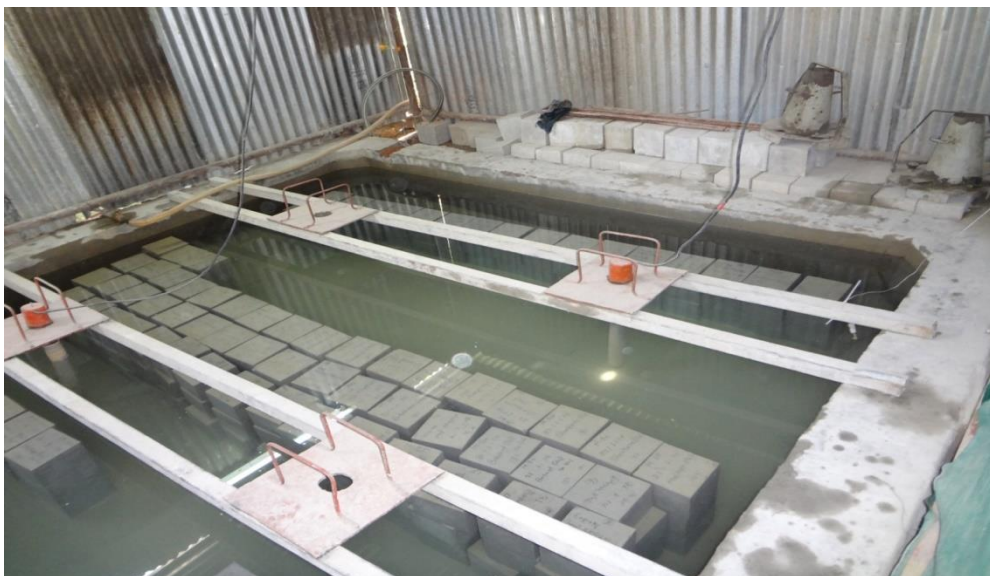
Fig:4.7 Test specimens being cured in curing tank
