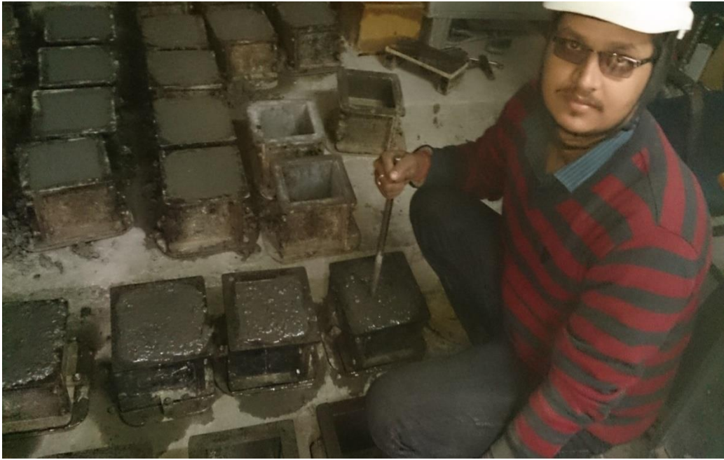
Fig:4.5 Compaction by Hand
