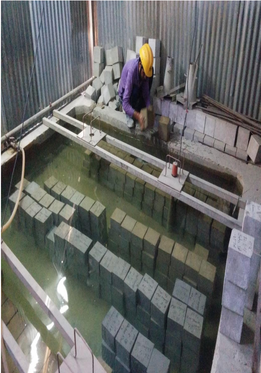
Fig: I.3 Curing of cubes in progress
