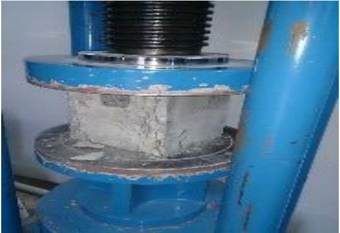
Fig:4.9 Cube Testing Compression Testing Machine
