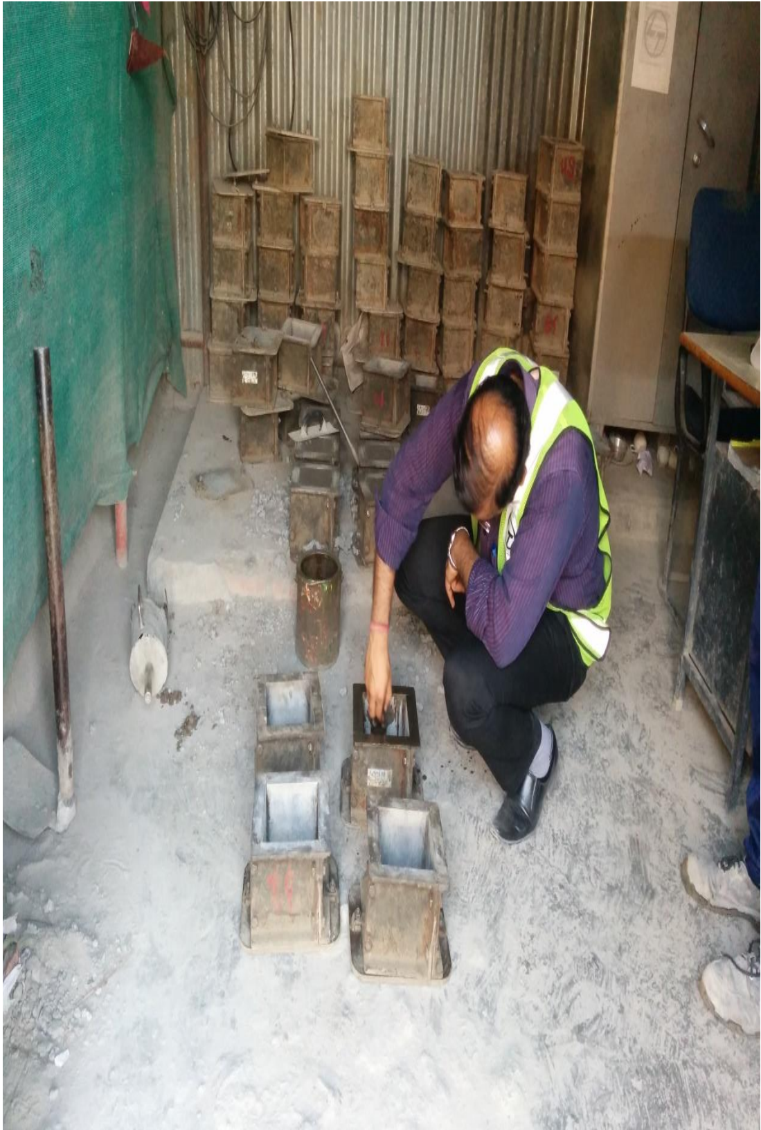
Fig: I.4 Work in Progress(Lubrication of cube moulds)
