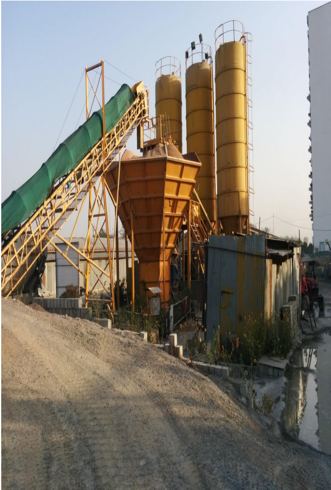
Fig: I.5 Ready Mix Plant in L&T Site
