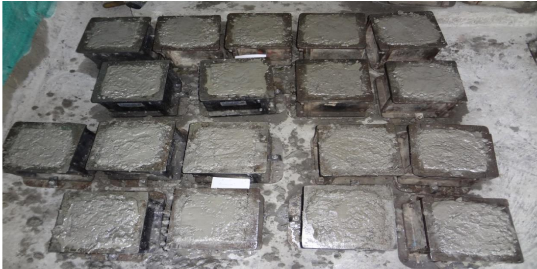
Fig:4.1 Concrete Casted in Moulds
