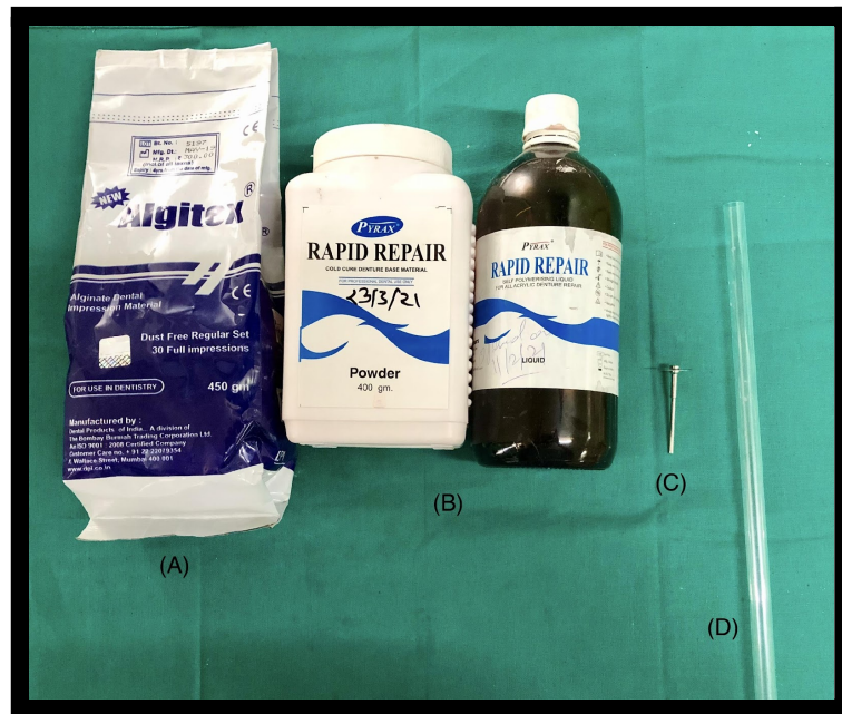
FIGURE 1: MATERIALS USED FOR FABRICATION OF MOULD (A) ALGINATE; (B) COLD CURE ACRYLIC RESIN; (C) DIAMOND DISK (D) PLASTIC CYLINDRICAL PIPE
