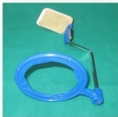
Assembly of Film Holder, mm GRID and IOPA Film
