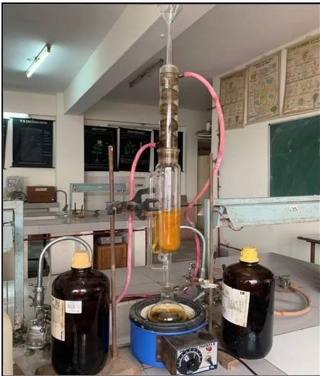
PLATE 3: EXTRACTION PROCESS BY OF CURCUMIN RIZOME BY SOXHLET APPARATUS
