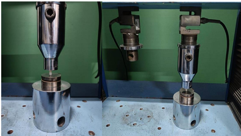
Figure 15: Compressive strength test with Universal testing machine
