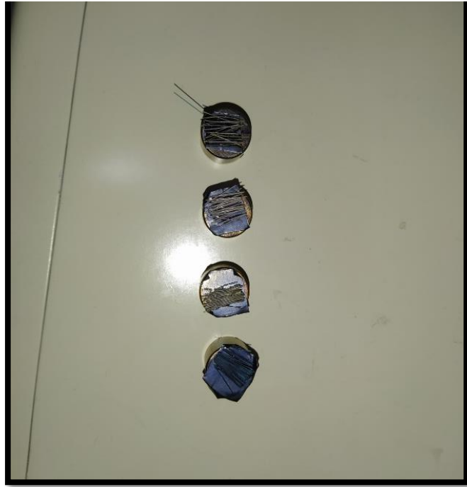
Figure7: Toothbrush Bristles Following Palladium-Platinum Coating
