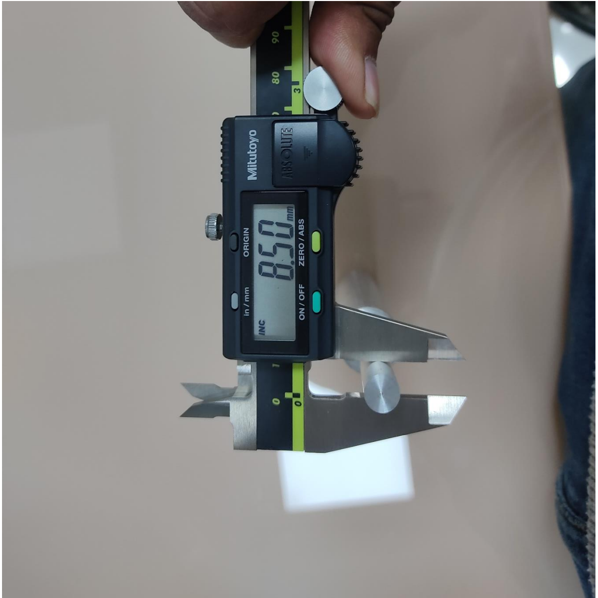
Figure 6.12 Final Diameter of the Workpiece
