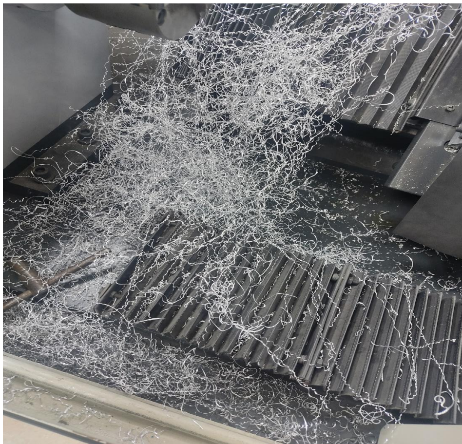
Figure 6.10 Chips formed in Turning Process
