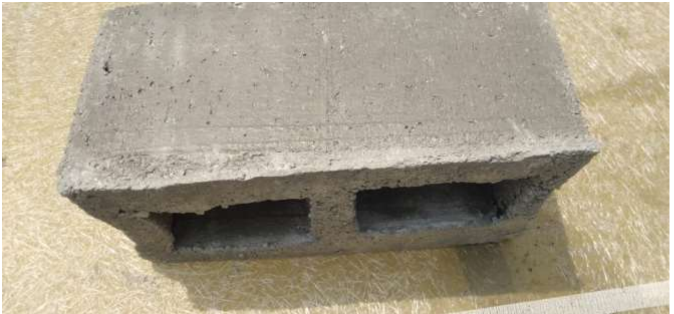
FIGURE 5.1-HOLLOW CONCRETE BLOCK MADE OF FLY ASH PARTIAL REPLACEMENT OF CEMENT
