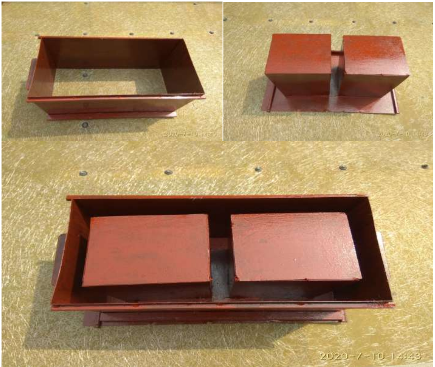
FIGURE 3.1 -MOULD USED FOR CASTING OF HOLLOW CONCRETE BLOCK
