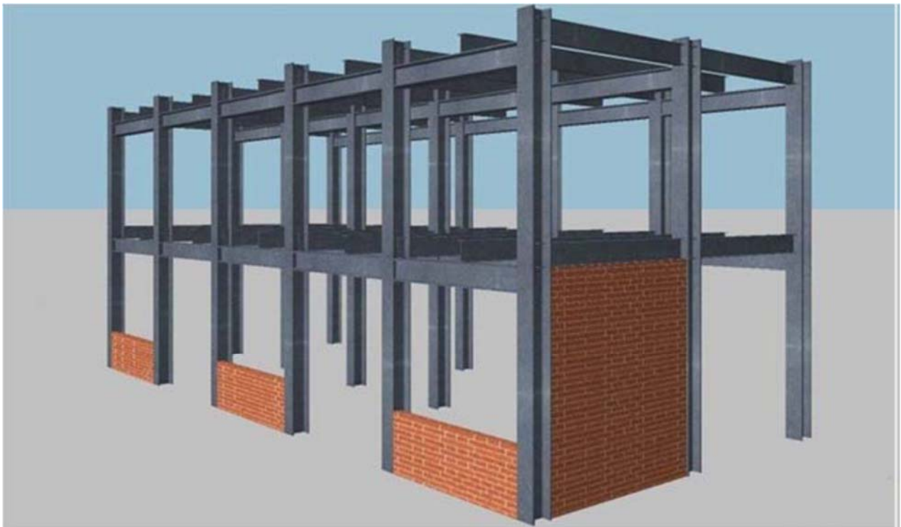
Fig. 1.1 An illustration of infill walls in framed structure
