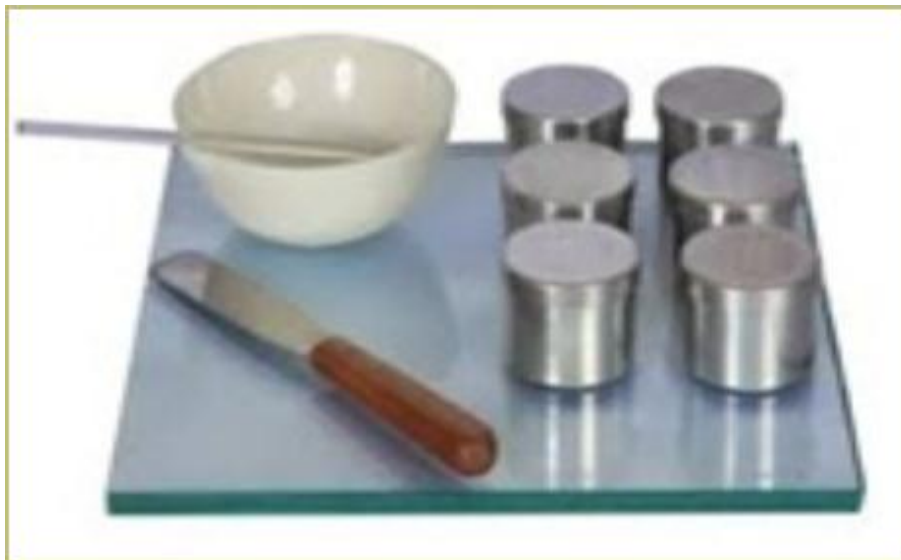
Fig.4.2.2(b): Plastic limit test equipment
