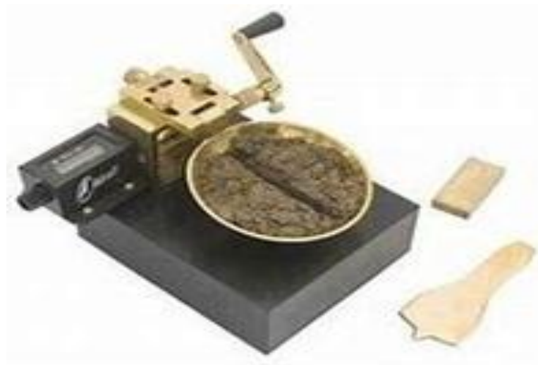
Fig. 4.2.2(a): Liquid Limit Test Device
