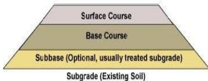
Fig 1.2.1.1: Layers of Flexible Pavement
