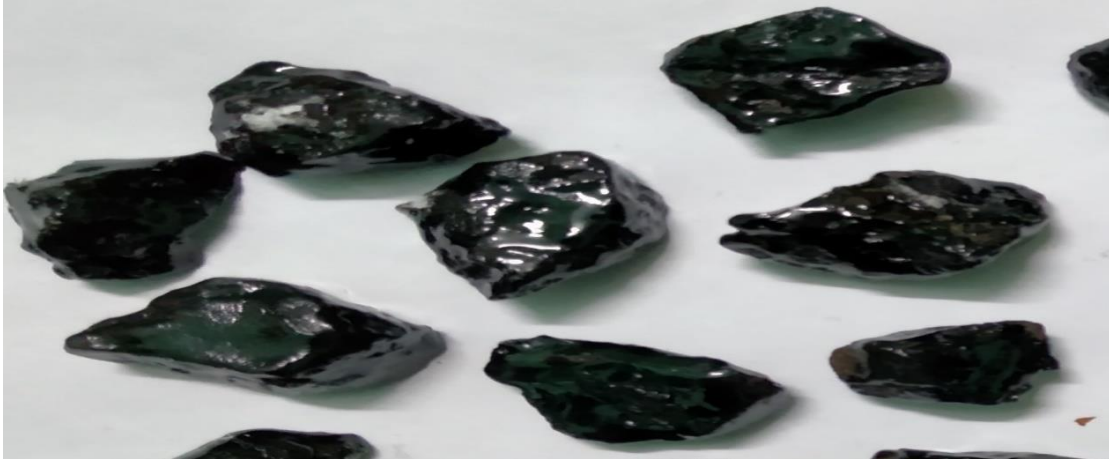
Fig 5.1.2.3 : Stripping after adding 1.0% Bitugrip in Boiling Water Test
