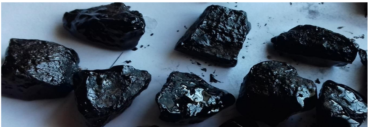
Fig 5.1.1.2: Stripping after adding 0.075% Zycotherm in Boiling Water Test
