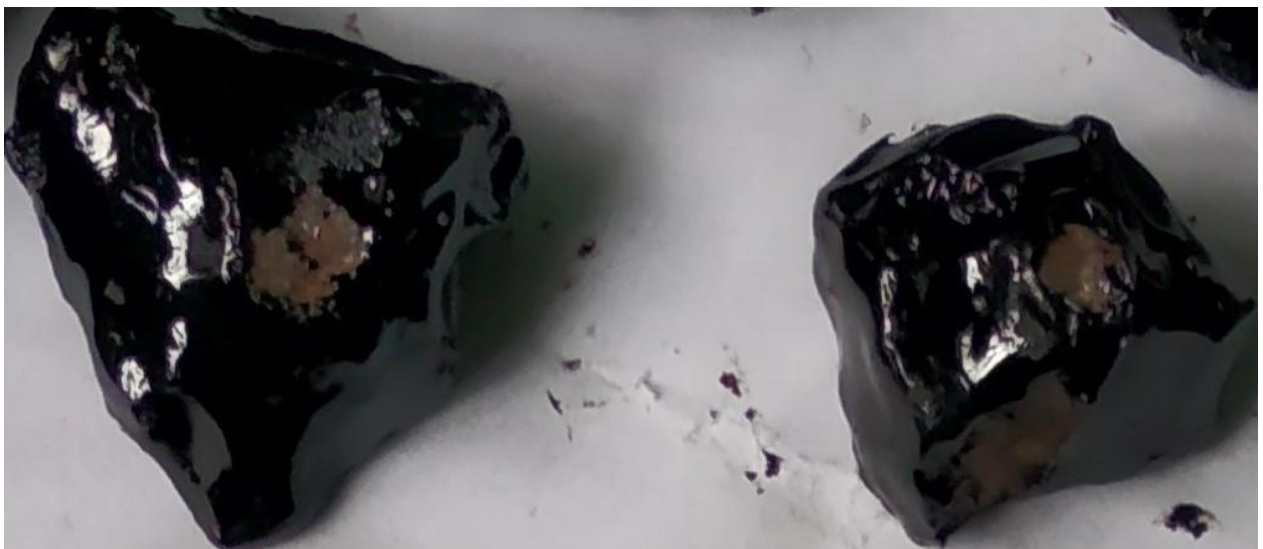
Fig 5.2.3.2: Stripping after adding 0.070% Wetbond-S in Stripping Value Test
