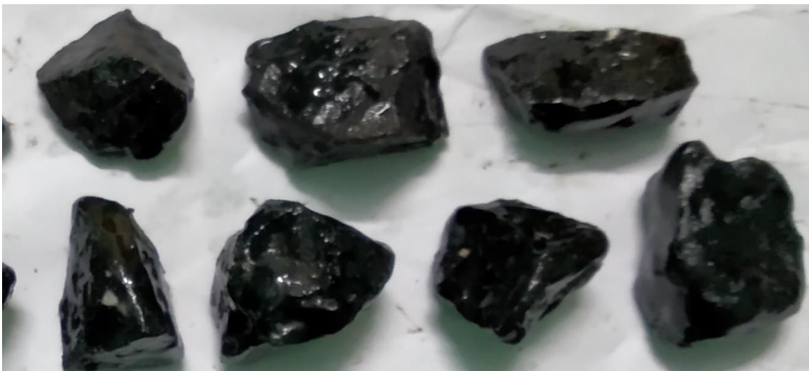
Fig 5.1.2.4: Stripping after adding 1.5% Bitugrip in Boiling Water Test
