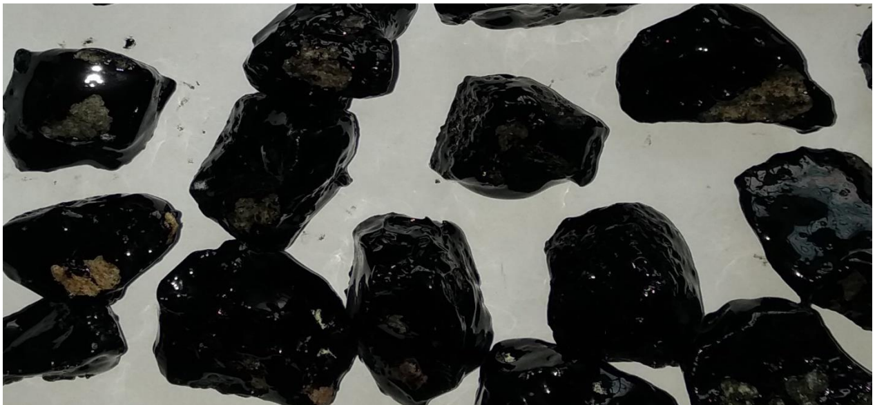
Fig 5.2.1.4: Stripping after adding 0.15% Zycotherm in Stripping Value Test
