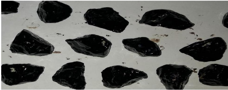
Fig 14: Stripping after adding 1.0% Bitugrip (Optimum) in Stripping Value Test
