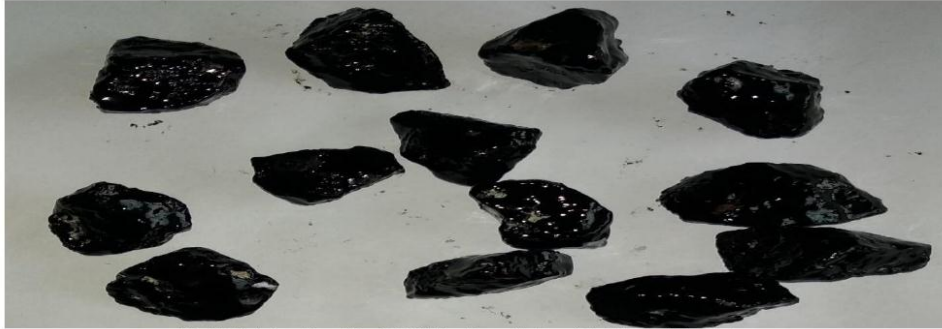
Fig 13: Stripping after adding 0.075% Zycotherm (Optimum) in Stripping Value Test
