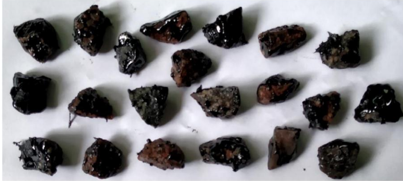
Fig 7: Stripping without adding any ASA in Boiling Water Test
