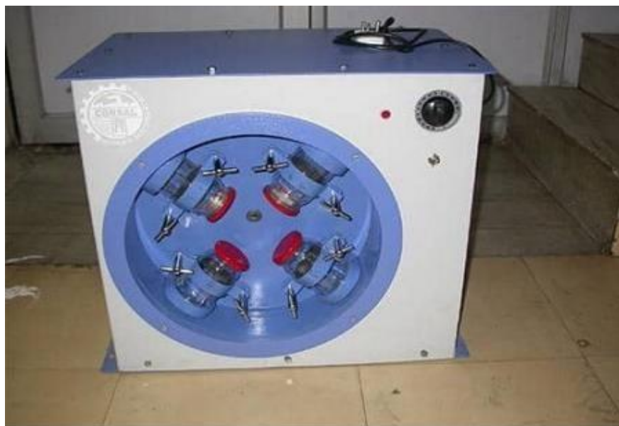
Fig 4.3.2: Test apparatus to mix Aggregate & Bitumen
