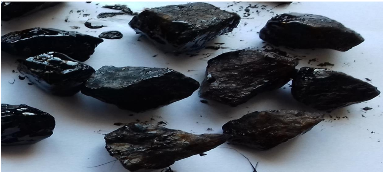
Fig 5.1.1.1: Stripping after adding 0.05% Zycotherm in Boiling Water Test
