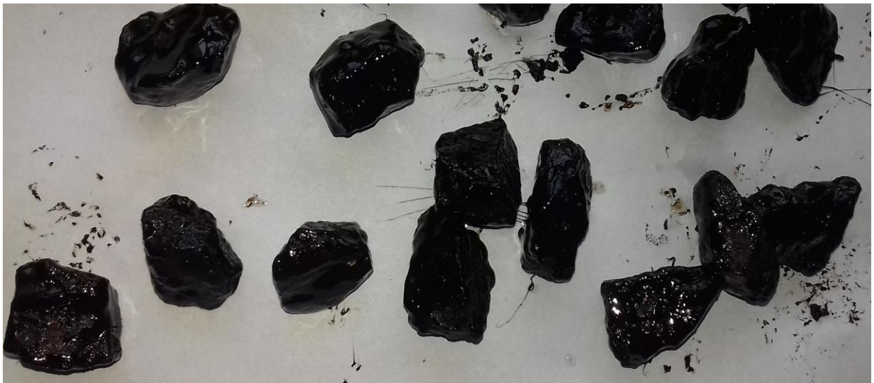
Fig. 5.1.3.2 Stripping after adding 0.07% Wetbond-S in Boiling Water Test
