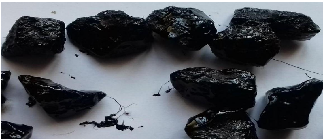
Fig 5.1.1.4: Stripping after adding 0.15% Zycotherm in Boiling Water Test
