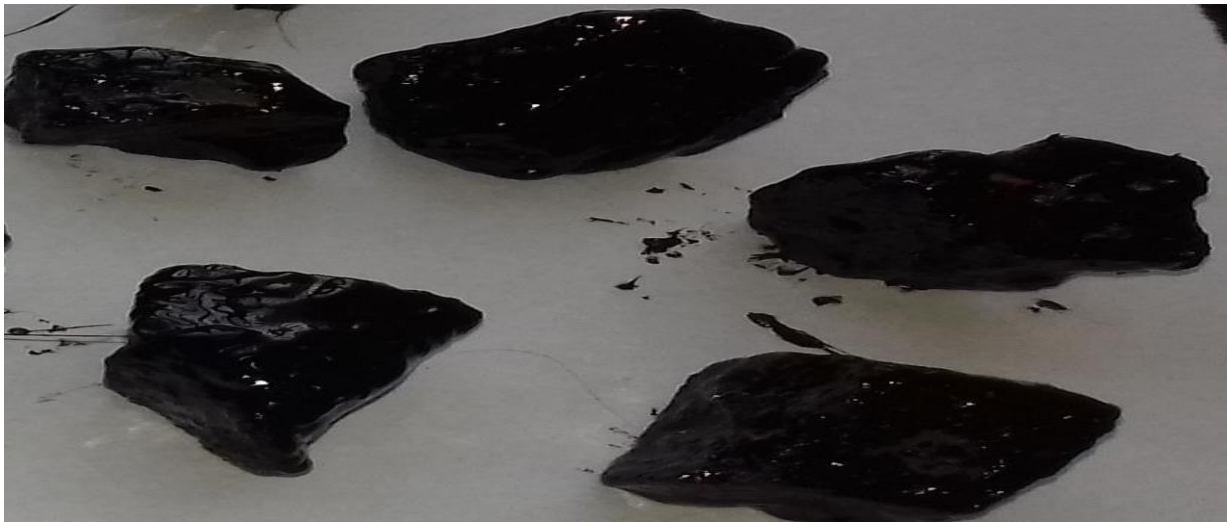
Fig 5.3.1: Stripping after adding Optimum Dose of Wetbond-S+Zycotherm in Boiling Water Test
