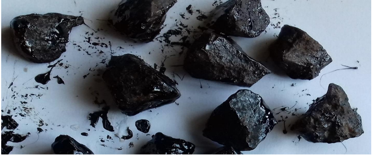
Fig 5.1.1.3: Stripping after adding 0.10% Zycotherm in Boiling Water Test
