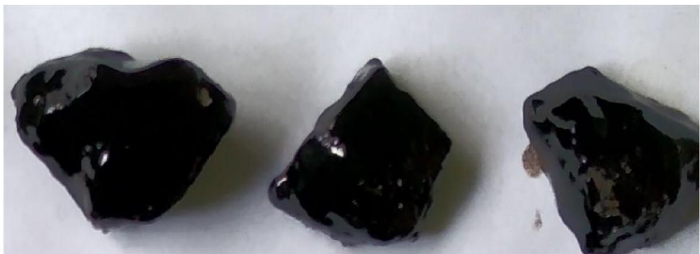
Fig 12: Stripping after adding 0.10% Wetbond-S (Optimum) in Stripping Value Test
