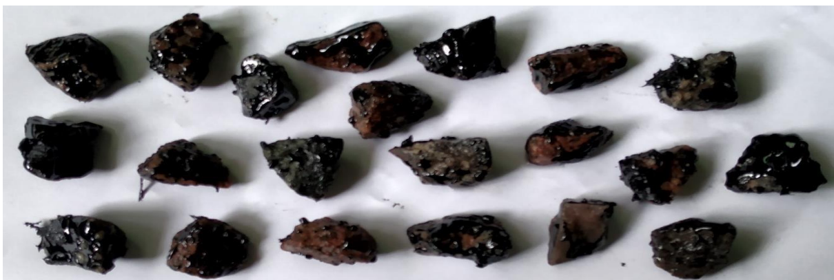
Fig 5.1: Stripping without adding Anti Stripping Agent in Boiling Water Test
