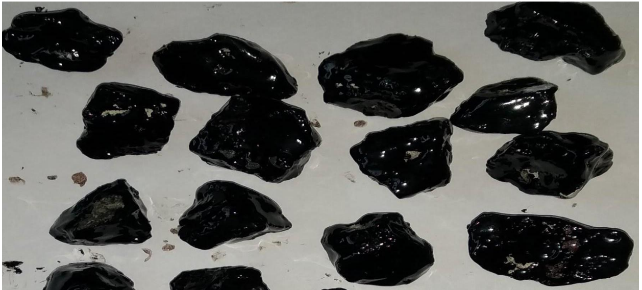
Fig 5.2.2.1: Stripping after adding 0.5 % Bitugrip in Stripping Value Test
