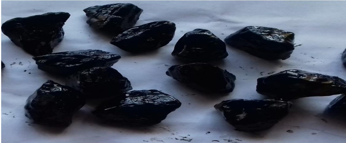
Fig 5.2.1.1: Stripping after adding 0.05% Zycotherm in Stripping Value Test
