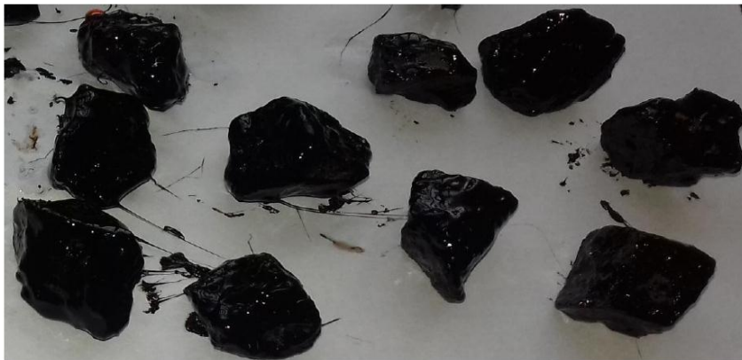
Fig 8: Stripping after adding 0.10% Wetbond-S (Optimum) in Boiling Water Test
