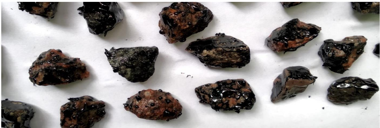
Fig 5.2: Stripping without adding Anti Stripping Agent in Stripping Value Test
