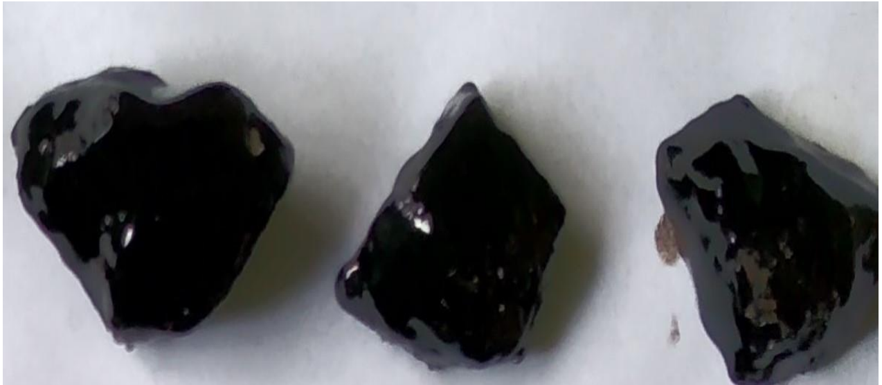
Fig 5.2.3.3: Stripping after adding 0.10% Wetbond-S in Stripping Value Test
