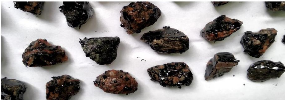
Fig 11: Stripping without adding any ASA in Stripping Value Test
