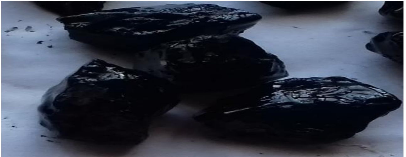
Fig 5.4.3: Stripping after adding Optimum Dose of Wetbond-S+Zycotherm+Bitugrip in Stripping Value Test
