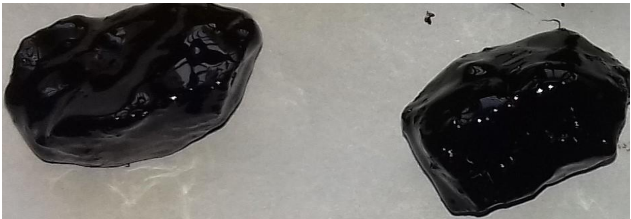
Fig 5.3.3: Stripping after adding Optimum Dose of Wetbond-S+Zycotherm+Bitugrip in Boiling Water Test
