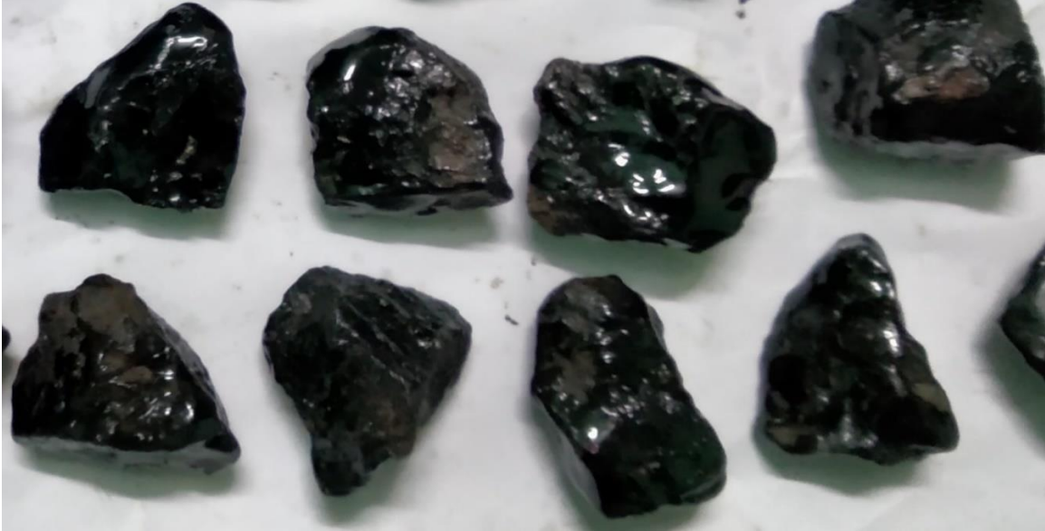
Fig 5.1.2.1 : Stripping after adding 0.5% Bitugrip in Boiling Water Test
