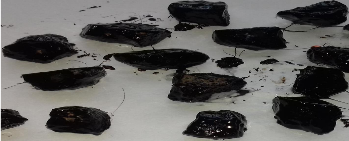
Fig 5.1.3.1: Stripping after adding 0.05% Wetbond-S in Boiling Water Test
