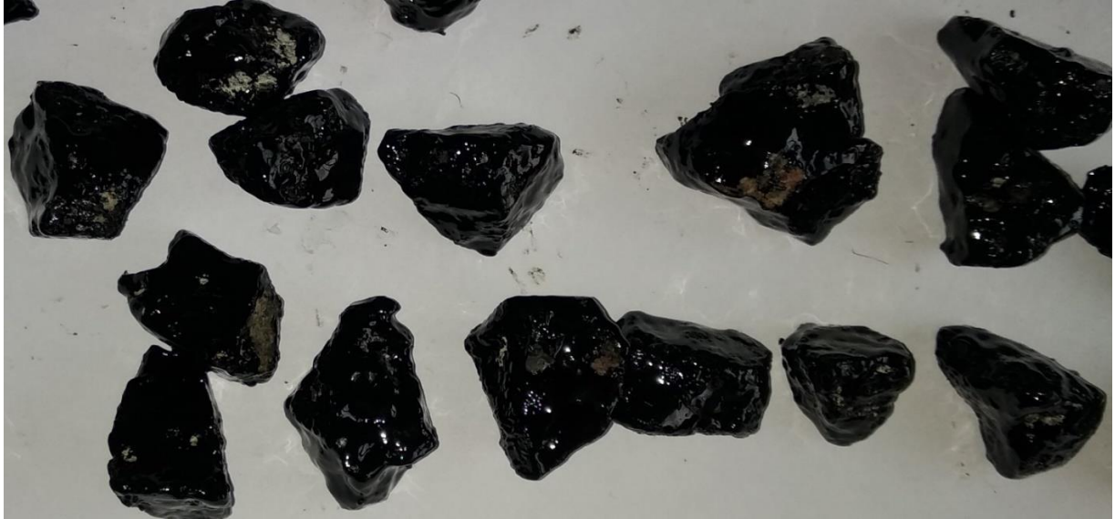
Fig 5.2.1.3: Stripping after adding 0.10% Zycotherm in Stripping Value Test
