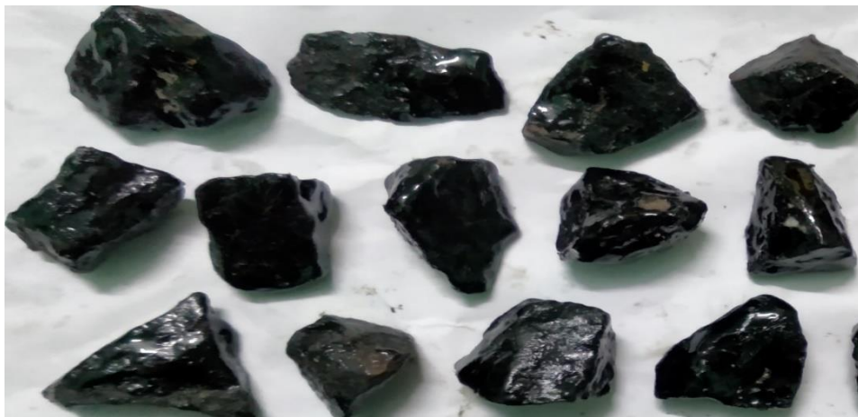
Fig 5.1.2.2: Stripping after adding 0.75% Bitugrip in Boiling Water Test
