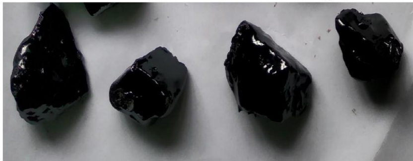
Fig 16: Stripping after adding optimum dose of Wetbond-S+ Zycotherm in Stripping Value Test
