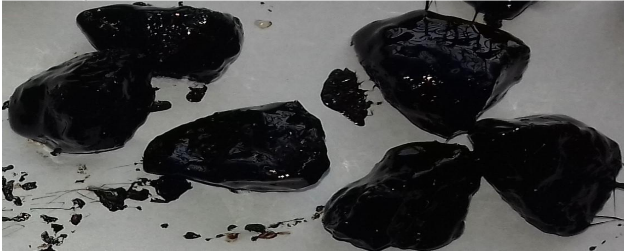
Fig 5.3.2: Stripping after adding Optimum Dose of Wetbond-S+Bitugrip in Boiling Water Test
