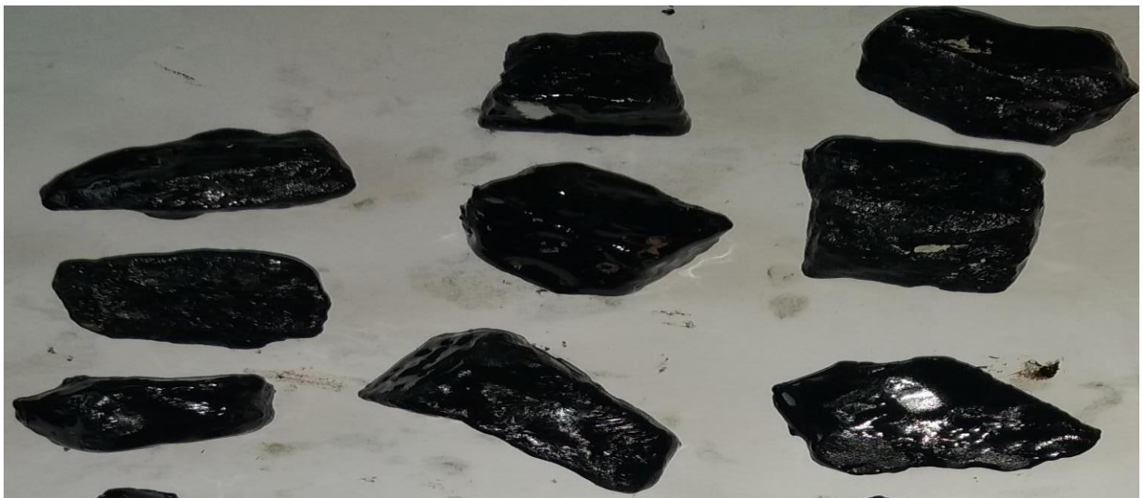
Fig 5.2.2.4: Stripping after adding 1.5 % Bitugrip in Stripping Value Test
