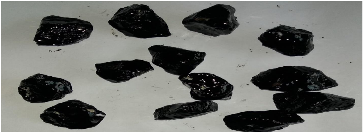
Fig 5.2.1.2: Stripping after adding 0.075% Zycotherm in Stripping Value Test
