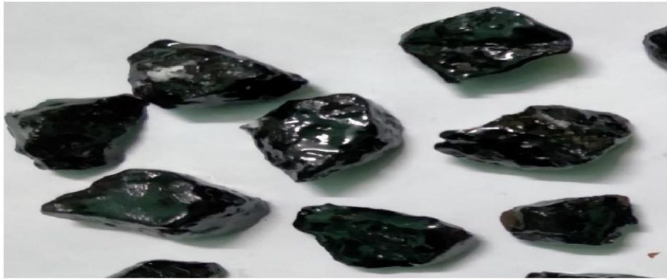
Fig 10: Stripping after adding 1.0% Bitugrip (Optimum) in Boiling Water Test
