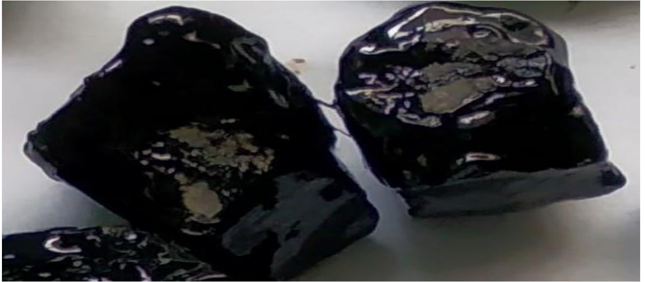
Fig 5.2.3.1: Stripping after adding 0.05% Wetbond-S in Stripping Value Test
