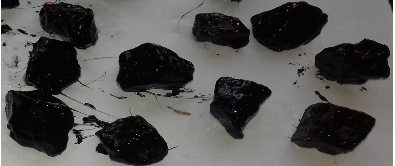
Fig: 5.1.3.3 Stripping after adding 0.10% Wetbond-S in Boiling Water Test
