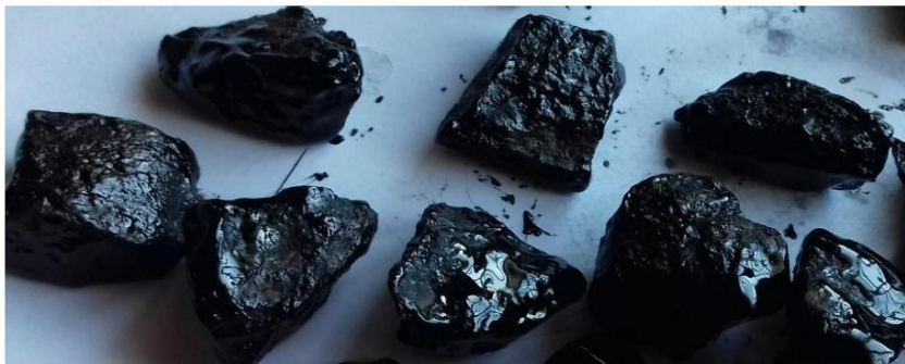
Fig 9: Stripping after adding 0.075% Zycotherm (Optimum) in Boiling Water Test
