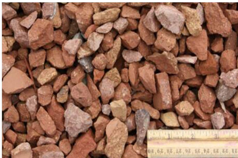
Figure 1.3 Capping Material-crushed bricks
