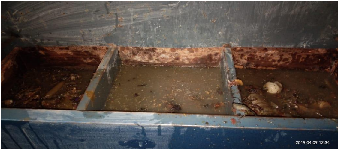
Fig. 4.9 Soil and Clays containers after five days of leachate addition
