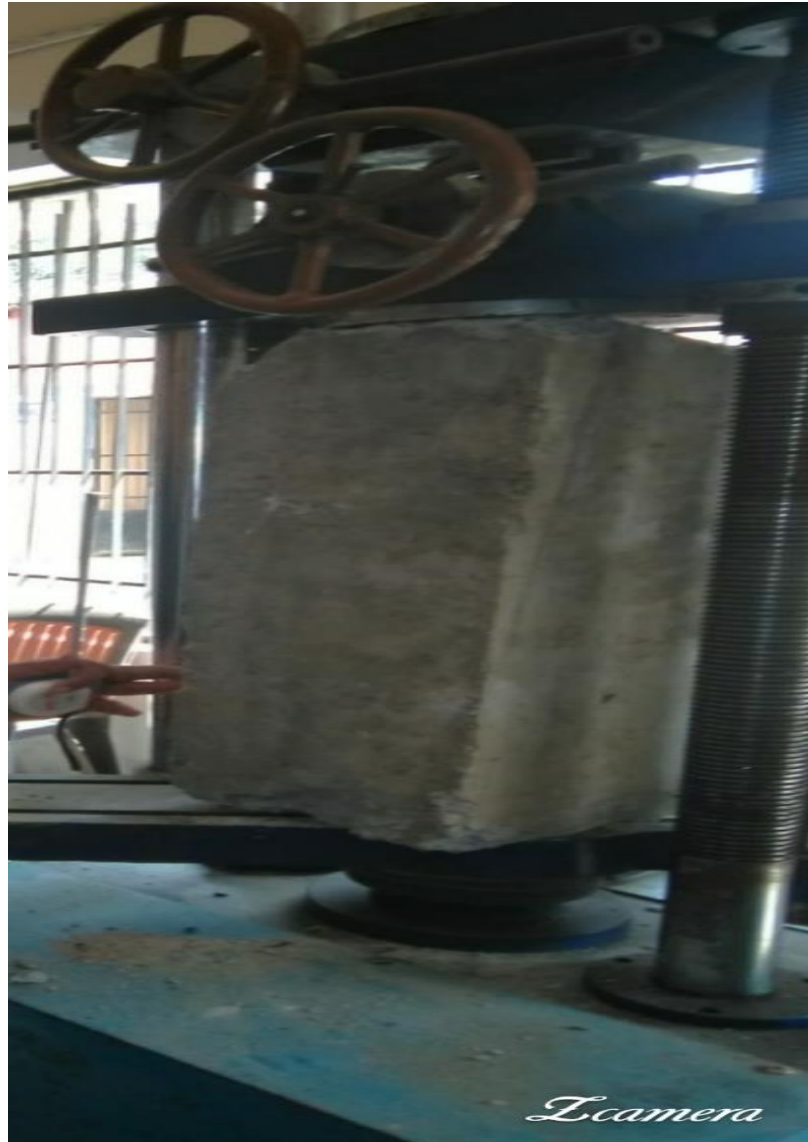
Fig 3.15 Column testing on UTM (universal testing machine)
