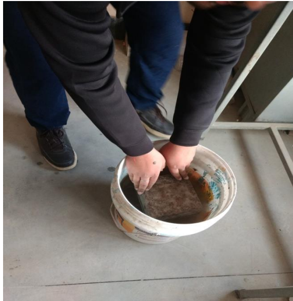
Fig 3.8 Curing of concrete cube
