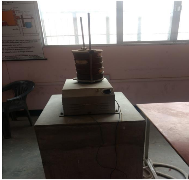
Fig 3.5 Sieve analysis of fine aggregate
