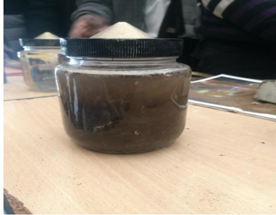
Fig 3.6 Testing of specific gravity of fine aggregate with Pycnometer
