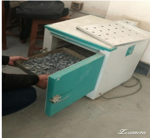
Fig 3.7 Drying of coarse aggregate in oven
