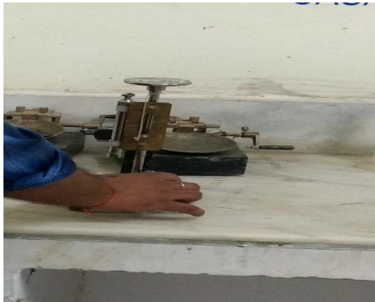
Fig 3.3 Testing of Initial and Final setting time with Vicat apparatus
