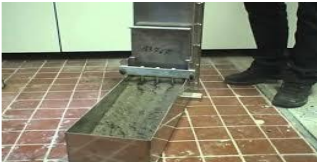
Figure: 3.5. L-box test
