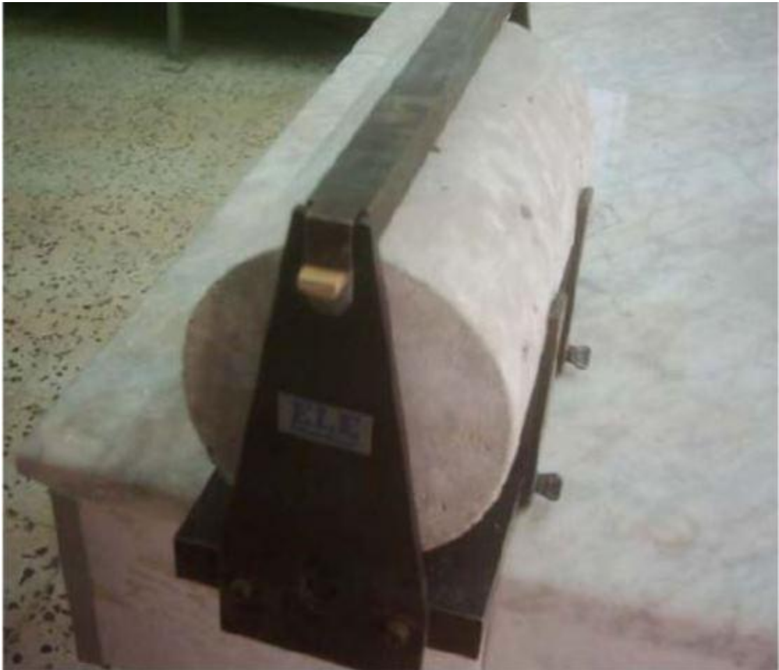
Figure: 3.8. Testing of Cylindrical Specimen under Split Tensile Strength Test
