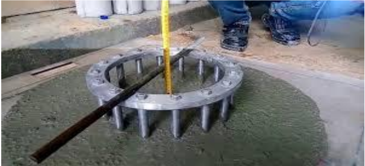
Figure: 3.3. J-Ring test
