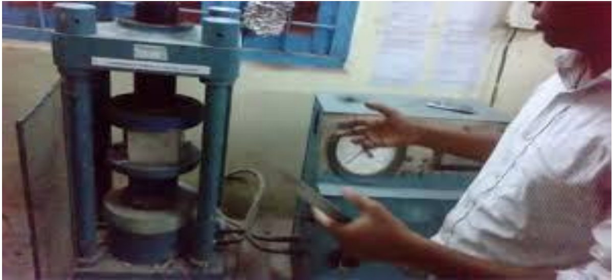
Figure: 3.7. Testing of Cube under Compression Testing Machine
