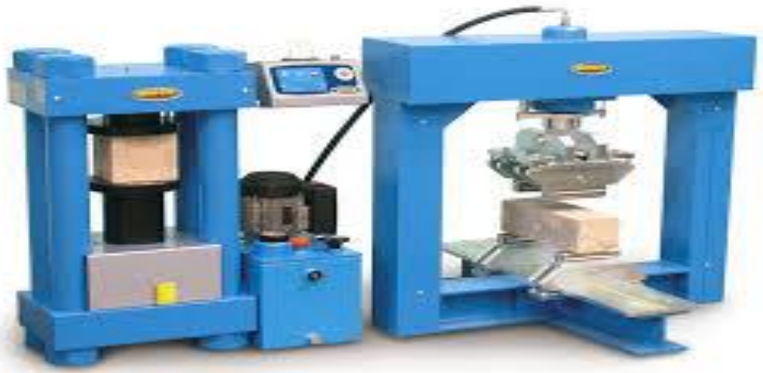
Figure: 3.9. Testing of specimen under flexure
