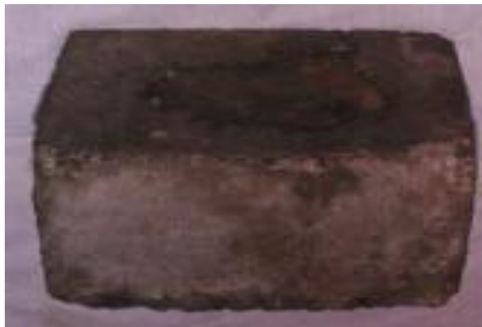
FIG.1 PRECAST CONCRETE STONE MASONRY BLOCKS
