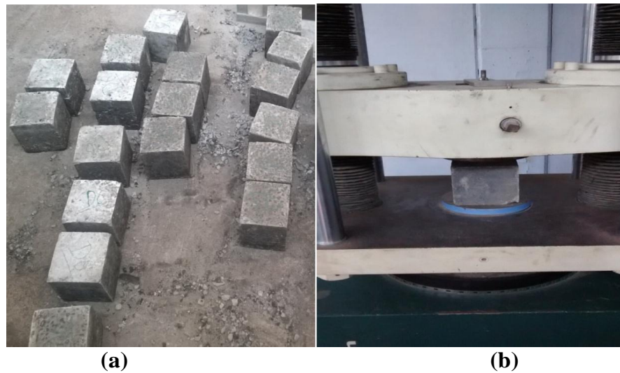
Figure 3.5: Demoulding and Testing of cube specimens
