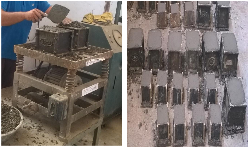
Figure 3.4: Casting of cube specimens
