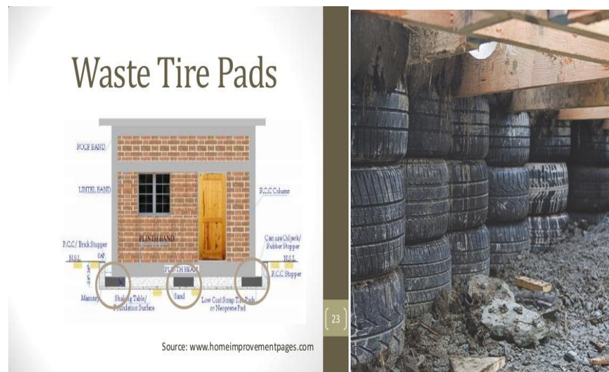
Figure 1.10- waste tire pads cross-section, Tire pads for retrofitting
