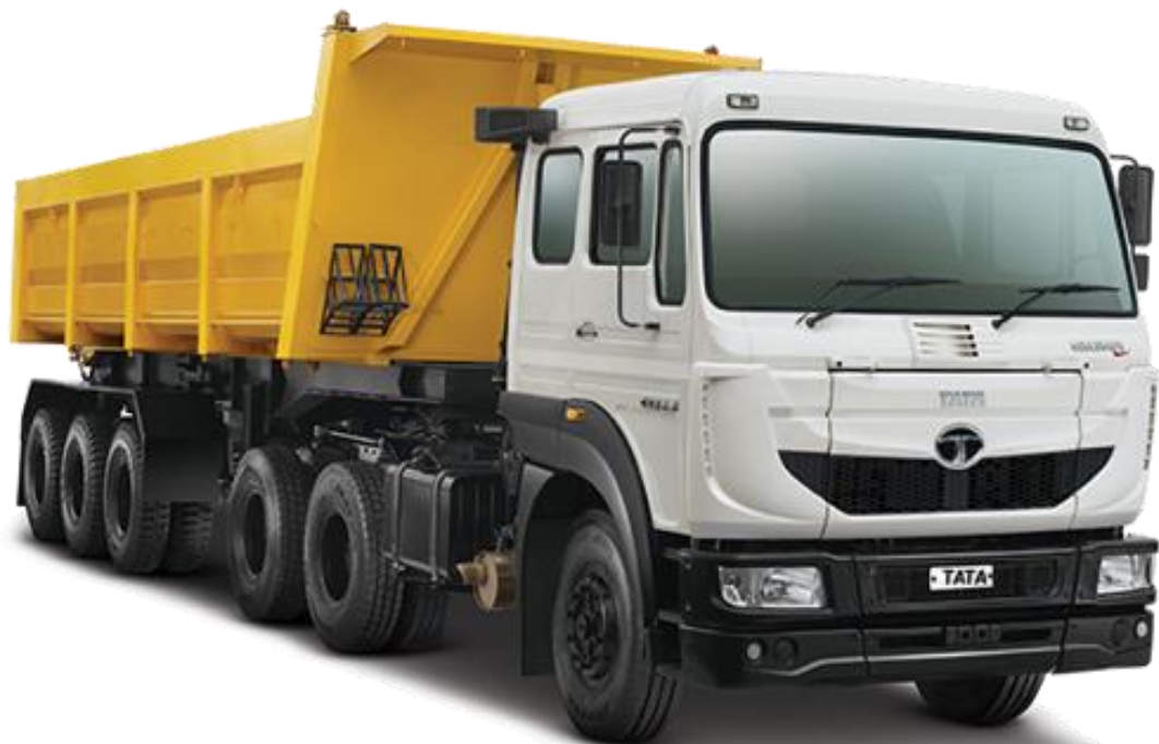
Figure 3.14 Tandem axle dual wheel
