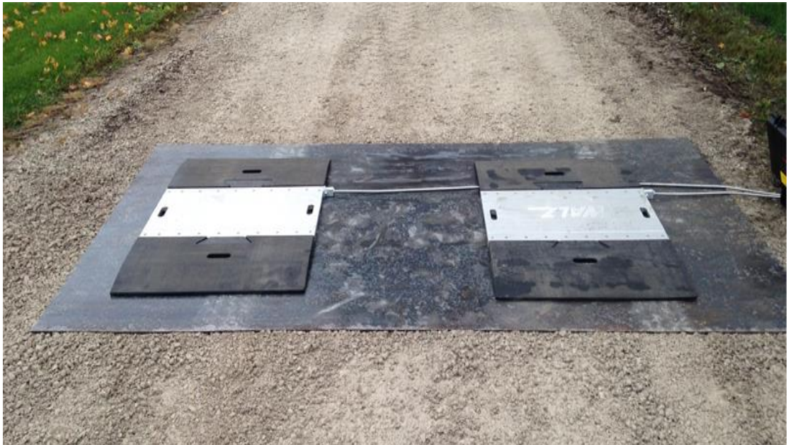
Figure 1.2 Weighing pads for weight in motion
