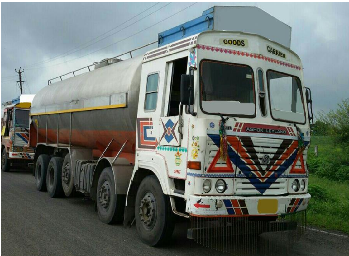
Figure 3.11 Tandem axle truck with convertible to tridem axle
