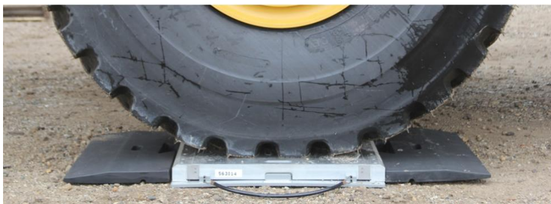
Figure 1.3 Weighing pads for weight in motion with truck load
