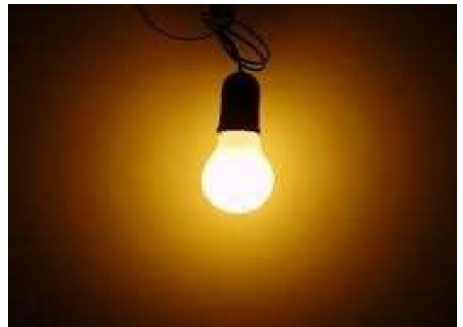
Incandescent lamps, are concentrated in the orange to red end of the spectrum.
