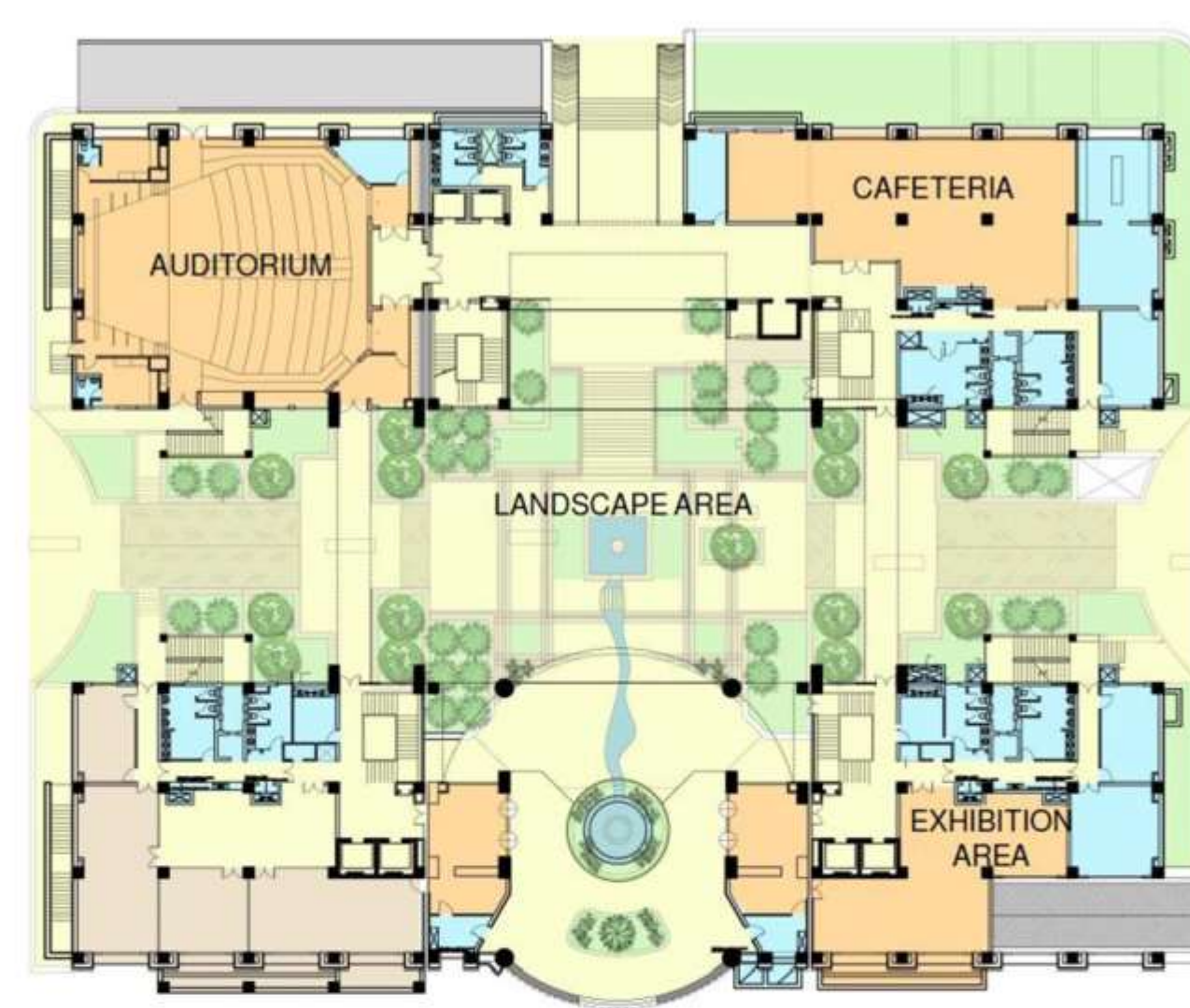
THE COURTYARD ALSO HELPS IN AIR MOVEMENT BESIDES BEING A SHADED INTERACTION SPACE
