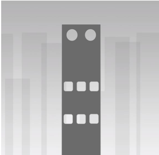
OPENINGS IN BUILDING REDUCE VORTEX SHEDDING
