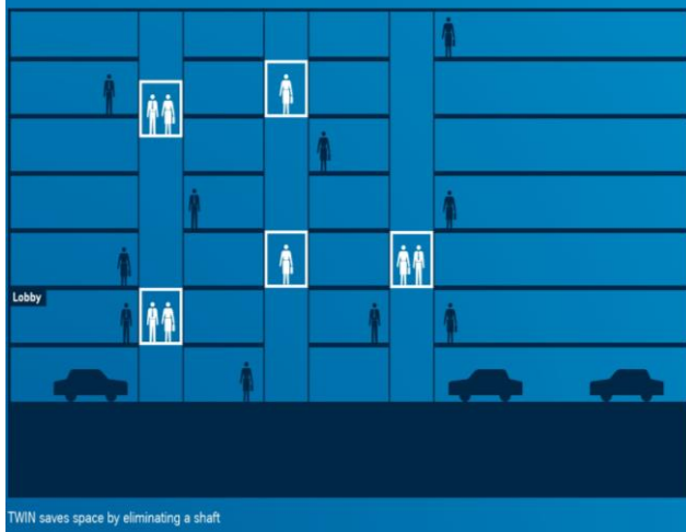
TWIN saves space by eliminating a shaft
