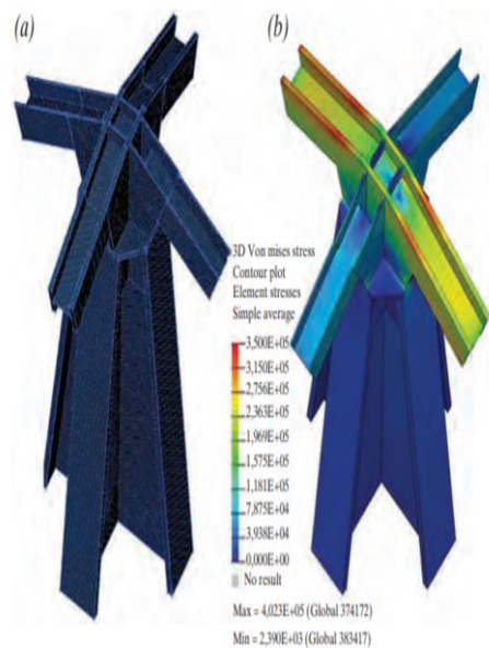
Fig. 3: Three-dimensional solid finite element analysis model of column pod top node connection: (a) three-dimensional finite element mesh of column pod top node; (b) finite element von Mises stress results of column pod top node (N/m 2 )
