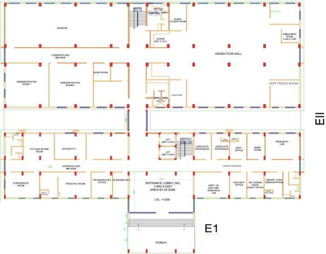
GROUND FLOOR PLAN OF MEDICAL COLLEGE
