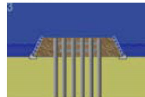
3 PERMANENT CONCRETE ARMOR UNITS PLACED AROUND ISLAND TO PROTECT IT FROM THE WAVES 1.5 M DIAMETER 45M DEEP PILES DRIVEN THROUGH ISLAND AND SEA BED BELOW TO
