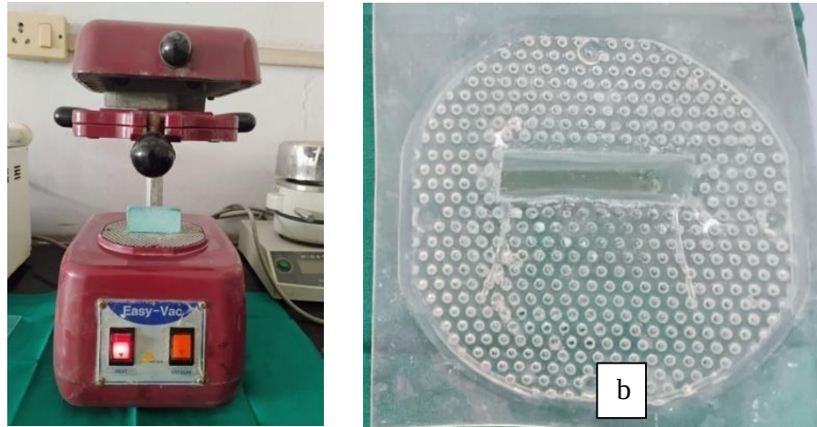
Figure 8 : a. Placement of stone block in thermo forming machine b.Mould of thermo forming sheet
