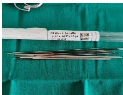
Figure 5 : Wires Used for measuring frictional force
