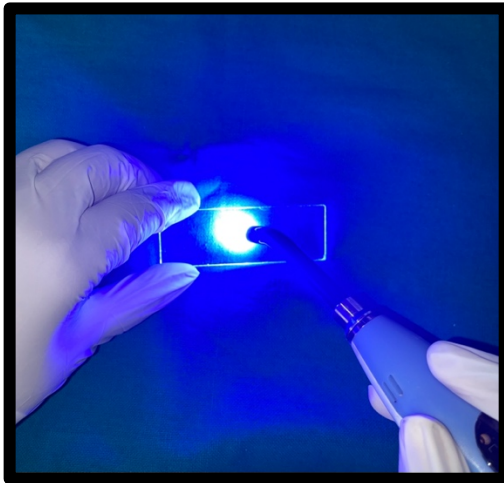
FIGURE 18: LIGHT CURING FOR 40 SECONDS
