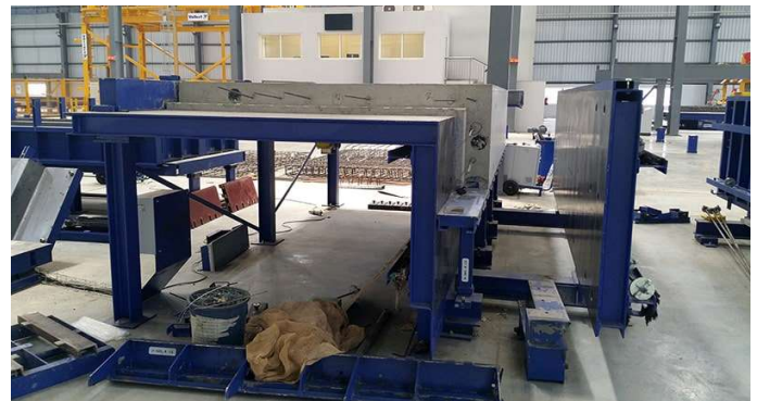
P 8. SPECIAL STATIONARY MOULD FOR L-SHAPED WALLS
