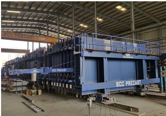
PIC. 10. BATTERY MOULD FOR VERTICAL PRODUCTION OF PRECAST WALL PANELS
