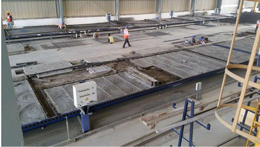
PICTURE 13. STEEL CASTING BEDS FOR PRECAST SLAB PRODUCTION
