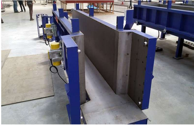
P 9. SPECIAL STATIONARY MOULD FOR PRECAST COLUMNS
