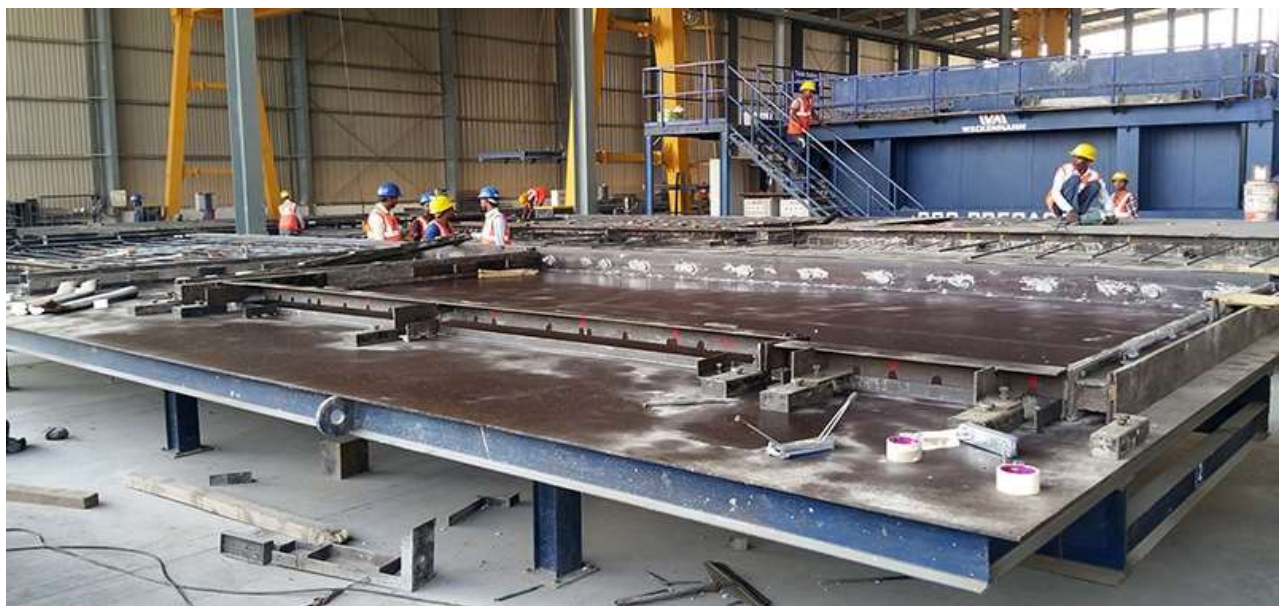
PICTURE 12. TILTING TABLES FOR HORIZONTAL PRODUCTION OF PRECAST WALL PANELS
