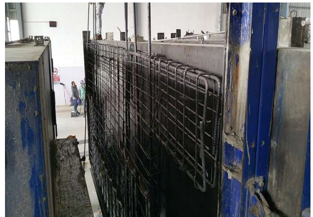
PIC.11. PRECAST WALL PANEL REINFORCEMENT CAGE INSIDE BATTERY MOULD SYSTEM
