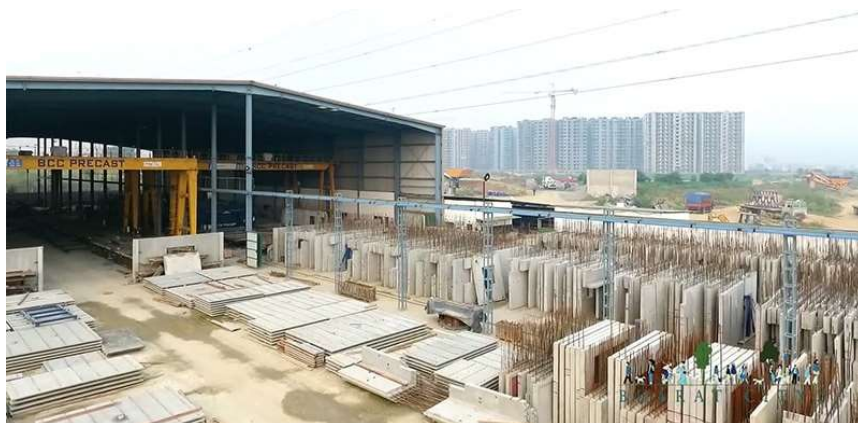
PICTURE 14. STOCKYARD FOR PRE-CAST ELEMENTS
