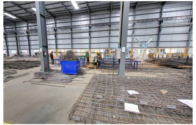
P 10. REINFORCEMENT WORKSHOP AND LATTICE GIRDER WELDING MACHINE
