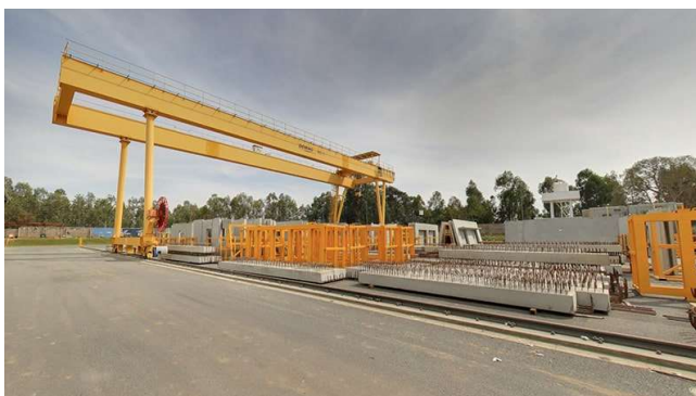
P 12. STOCKYARD FOR STACKING OF PRECAST ELEMENTS
