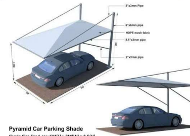
Pyramid Car Parking Shade Shade Size For 1 car (6M) x 3M (M) x 9.5M
