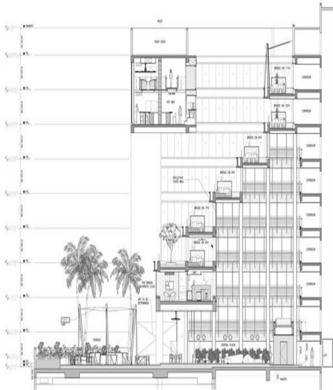
SECTION 1-SECTION THROUGH TERRACE AND CENTRAL PLAZA
