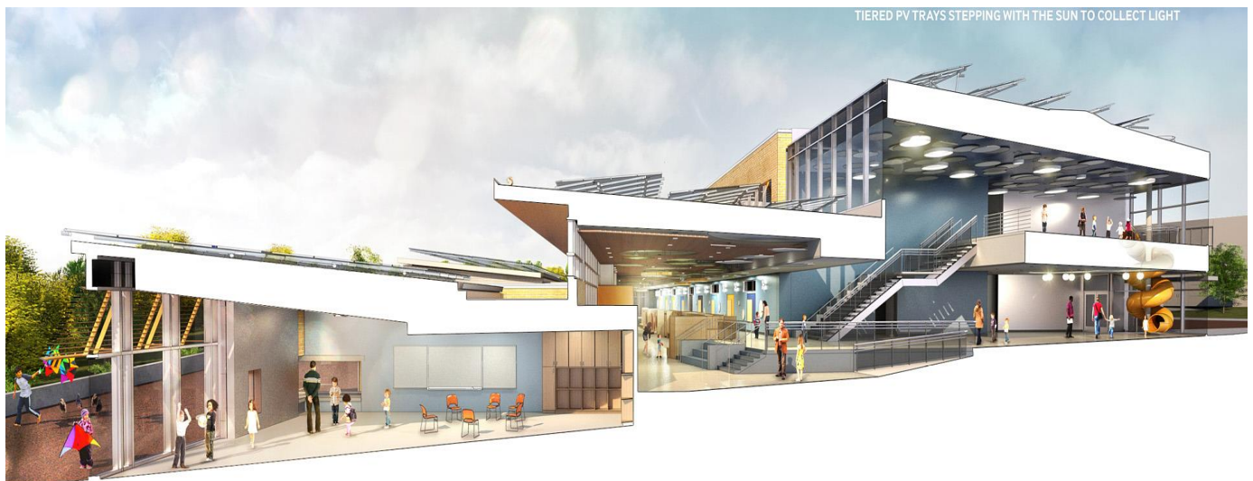
SECTION OF TIERED PV TRAYS STEPPING WITH THE SUN TO COLLECT LIGHT
