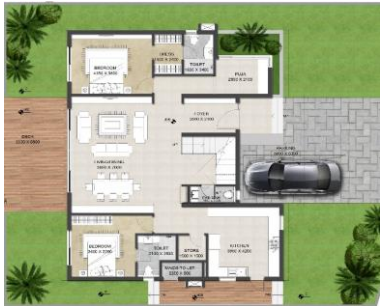
EAST FACING GROUND FLOOR PLAN
