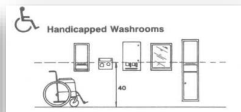
Mounted heights for bathroom accessories
