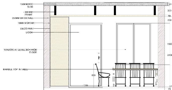
SECTIONAL ELEVATION BB'
