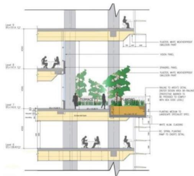
Figure 3.A.2.19: Detail of Green Ramp, Solaris, Singapore
