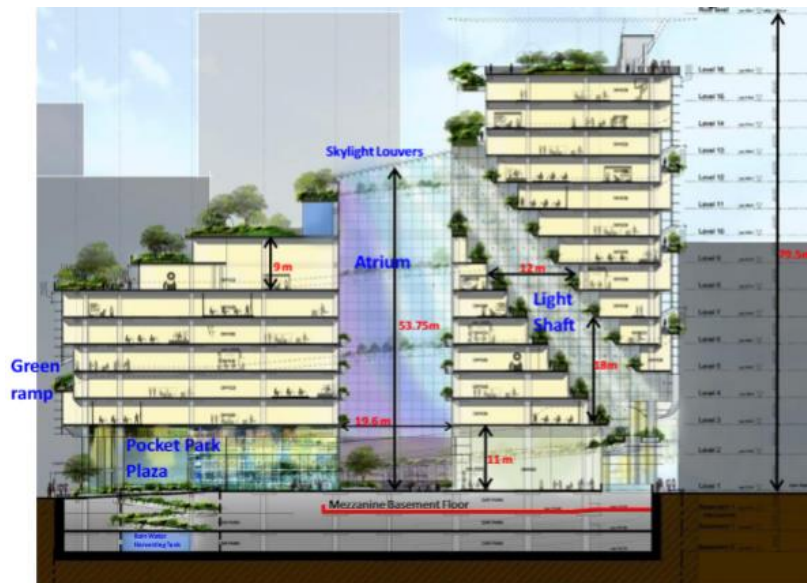
Figure 3.A.2.18: Building Section, Solaris, Singapore
