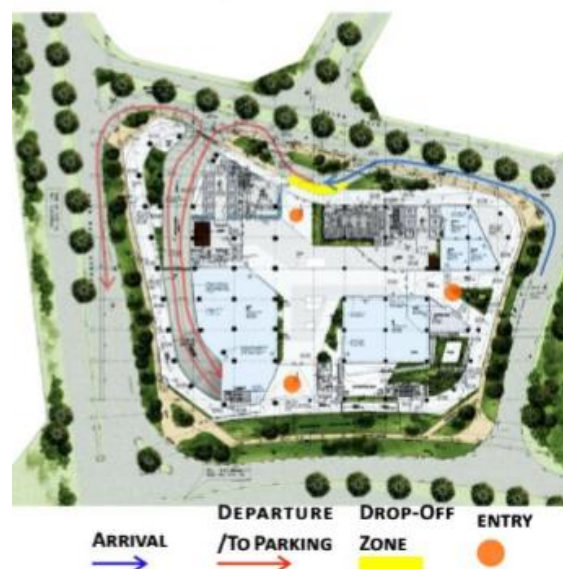
Figure 3.A.2.3: Circulation Plan, Solaris, Singapore (source: https://issuu.com/hardeepsingh8/docs/1 )
