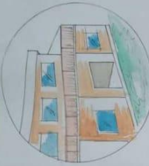
VIEW SHOWING NORTHERN GLASS FACADE TO LET IN GLARE FREE LIGHT AND PERGOLA FOR SHADING
