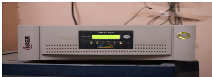
Figure 3.1(f) Start solar inverter through solar panel and grid Source : Author
