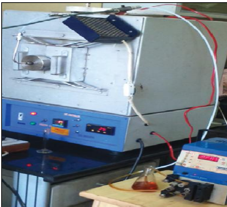
Figure 2 showing the external image of CVD machine during reaction
