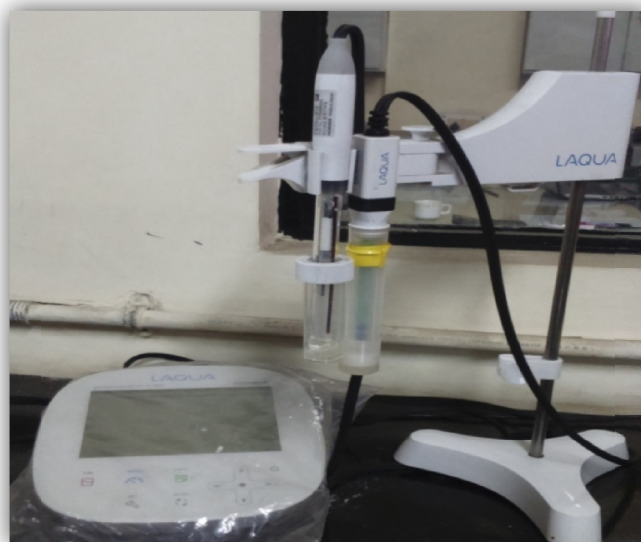
Figure 3.10: Ion Meter For measurement of Electrical conductivity
