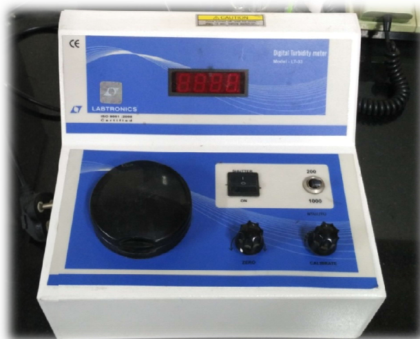
Figure 3.9: Determination of turbidity by turbidity meter.
