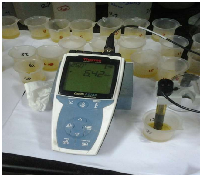
Figure 3.4: Showing fluoride analysis in groundwater samples in the laboratory
