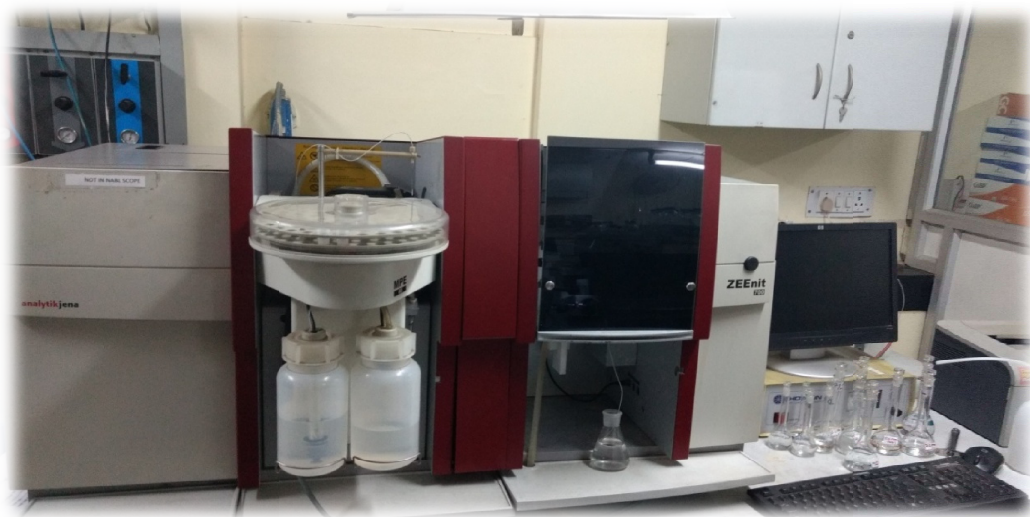
Figure 3.11 Atomic absorption spectrophotometer
