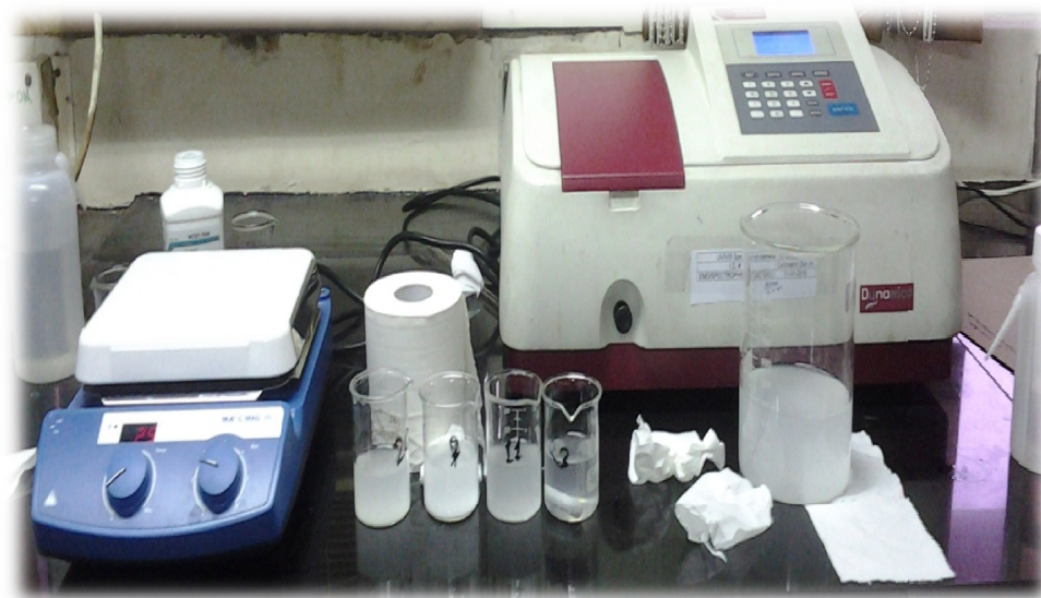
Figure 3.8: Determination of sulphate through spectrophotometer.
