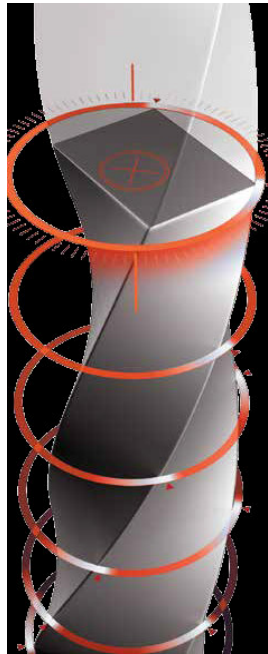
Figure 1.15. Protaper Next File design showing rectangular cross section and mass of rotation being offset.
