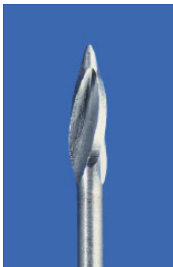
Figure 1.17. Cutting Head of Gates Glidden Drill.
