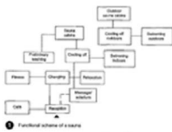
1 Functional scheme of a sauna
