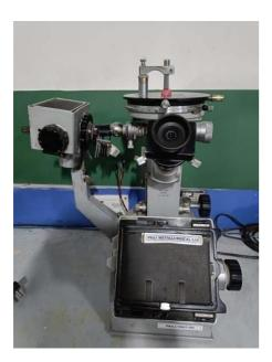
Fig 26 - Vicker's Microhardness tester
