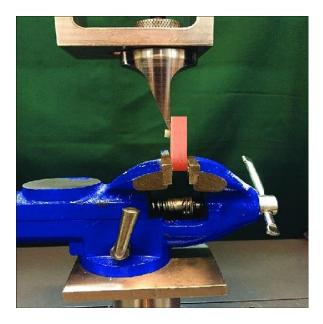
Fig 28 – Microshear Bond Strength Testing using Universal testing machine
