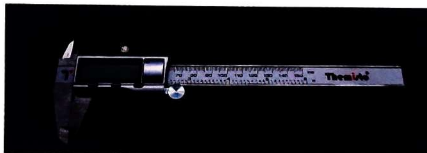
Figure 3: Themisto TH-M61 Digital Vernier Calliper
