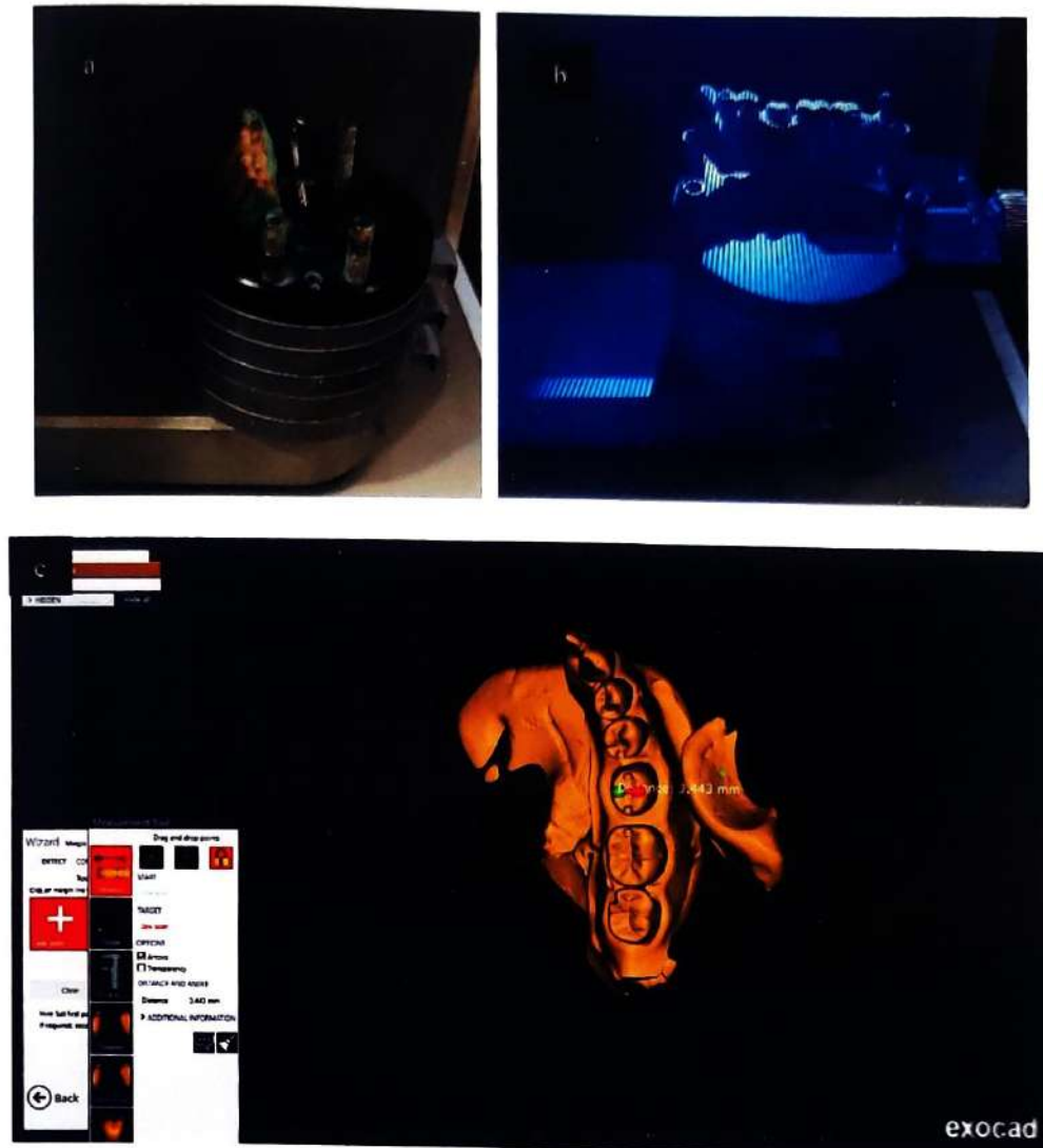
Figure 15: Die-stone cast scanning with Extraoral Scanner (MEDIT, Korea)
