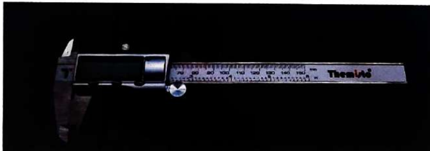
Figure 3: Themisto TH-M61 Digital Vernier Calliper
